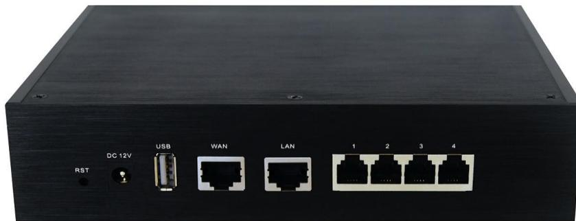
Figure 2-5 Rear view of MUC2008
